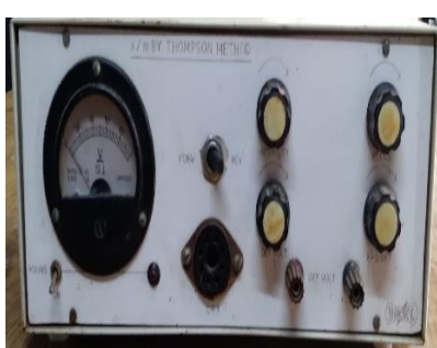
9. e/m Thomson experimental set-up.
